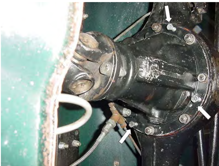
The differential-removing jacking bolts ready to work
