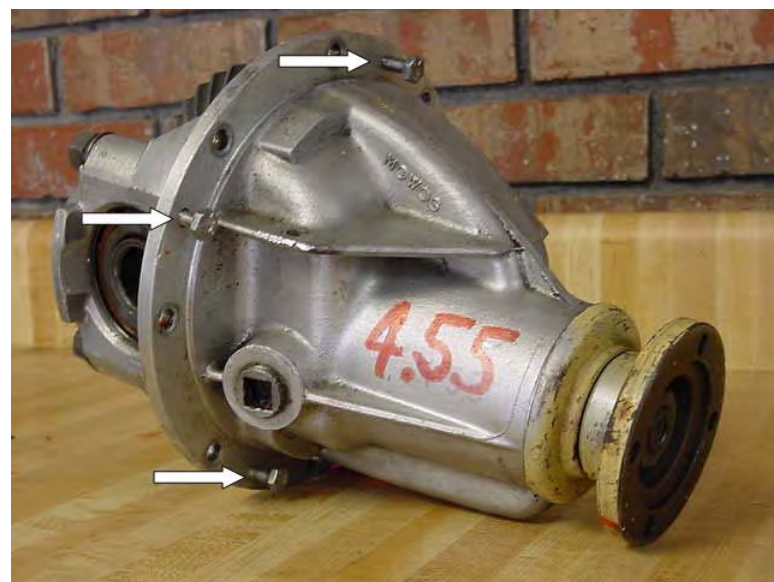
The placement of three of the four jacking bolts on the differential flange
